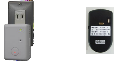
Fig. 4. Power meter and Transmitter of the ultrasonic positioning sensor
